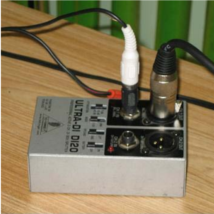
Image 3.5 Small mono jack for phono (kleine Klinke auf Cinch in German) for the audio from the distance to be transmitted audible in the room. This was especially important for the video conferencing with Jon Husband, Harald Jarcke and Kevin Wheeler who joined live online.
