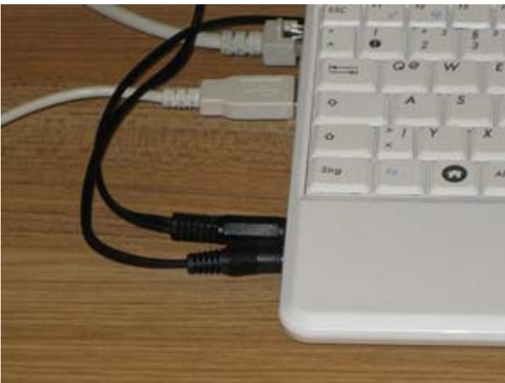
Image 3.2 Close up of mic in and audio out and USB to camcorder.
